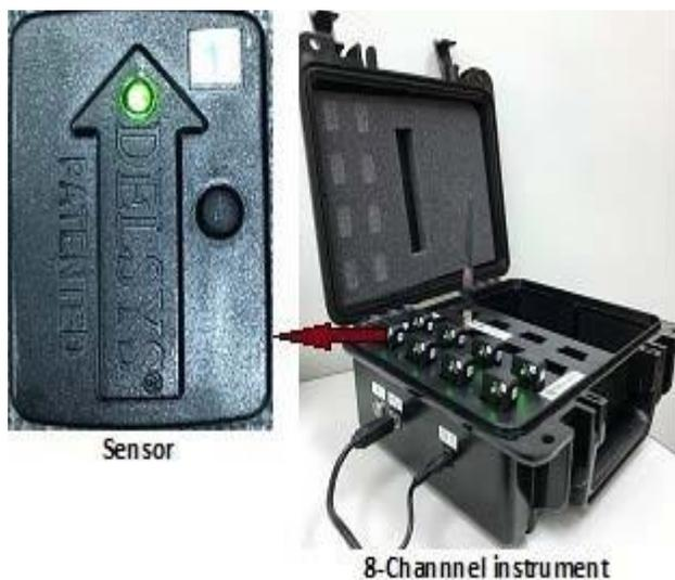
Figure 4 DELSYS Trigno Wireless EMG instrument showing the base station and a sensor.
