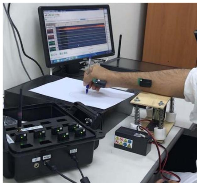
Figure 7 Experimental set up to record EMG and accelerometer signals from muscles during the writing task.
